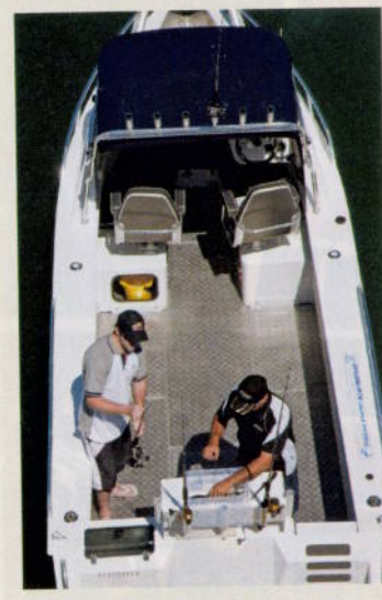
The 6700 Cabin's cockpit is a spacious workshop for bluewater fishing. Note the wide side decks and checkerplate deck — a carpeted deck is optional.
