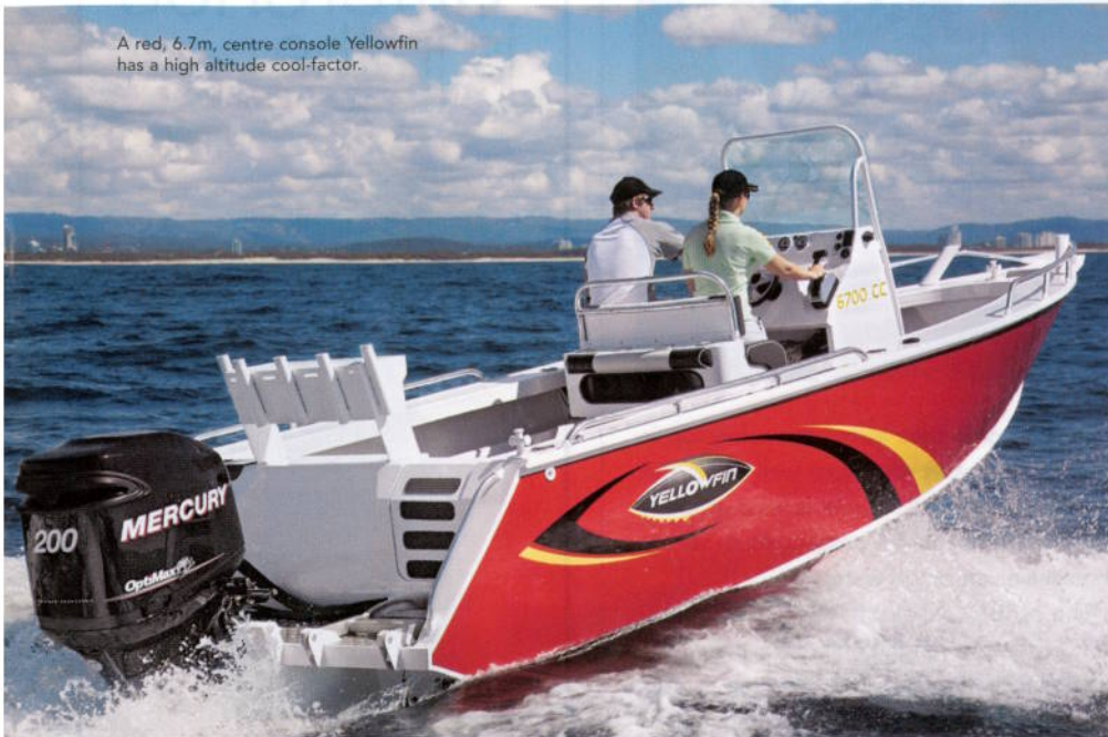
A 20-degree deadrise at the transom and fairly fine bows ensure a smooth offshore ride.
