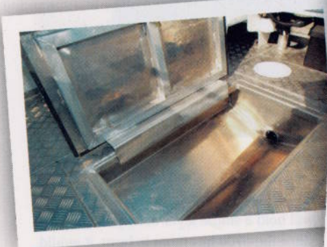
Clockwise from top: Under the hammer, the big Yellowfin 6700CC is a smart performer, getting to the fishing grounds quickly and efficiently; Close-up of the helm seat frame, housing the icebox; Raised forward platform has underfloor storage for safety gear; The cockpit's 135lt killtank drains to the transom and not the bilge.
